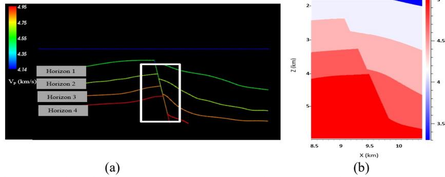
Figure 2. (a) A 2D cross section of the model which shows the horizons and the fault plane. The white box is the area of the study for PSDM simulation. (b) The reflectivity of the model in the area of the investigation.
