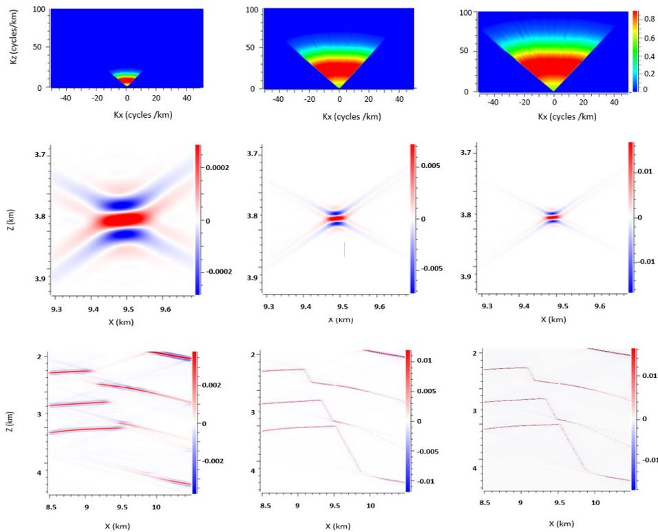
Figure 3. The PSDM filters (top row), PSF (middle row) and the PSDM images (bottom row) for Ricker zero-phase source wavelet 20 Hz (left column), 60 Hz (middle column), and 80 Hz (right column). The 20 Hz source wavelet has low resolution on the PSF, and the fault plane cannot illuminate on the PSDM image.
