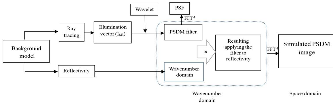
**Figure 1. The flowchart of PSDM image generation. The simulated PSDM image is calculated by the inverse Fourier transform of multiplication of reflectivity and PSDM filter in the wavenumber domain.**
