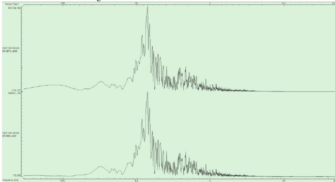
**Figure 3.** Spectra of the teleseismic event Mw 5.2 near cost of Western Turkey, recorded by CME-6211 broadband seismometer (upper trace) and Trillium 120 (lower trace).
