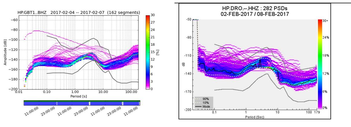
**Figure 4.** Comparison of the spectra recorded at quiet time period. Left – CME-6211 120 sec seismometer. Right – Trillium 120.
