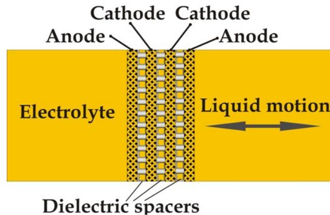
Figure 1. Molecular-electronic transfer cell.
