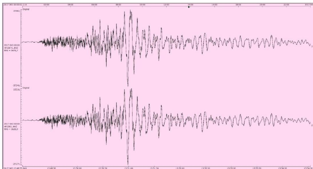
Figure 2. Teleseismic event Mw 5.2 near the cost of western Turkey, recorded by CME-6211 broadband seismometer (upper trace) and Trillium 120 (lower trace).
