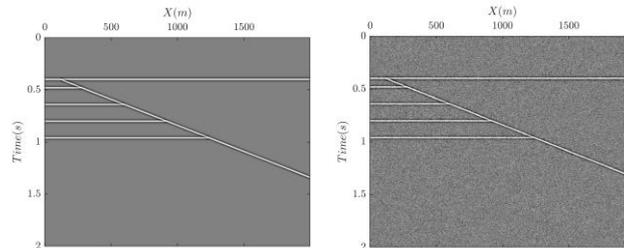
**Figure 2.** Wedge model example. (Left): noise free section. (Right): noise contaminated data.
