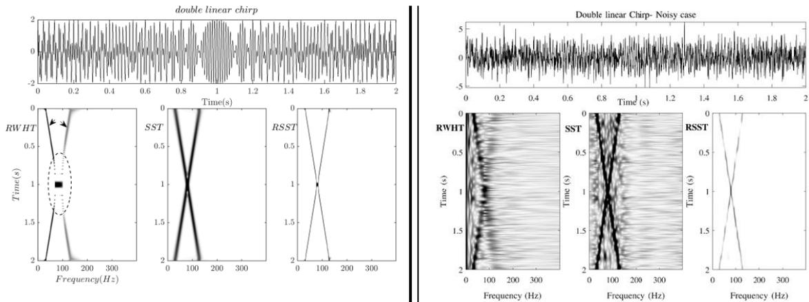
**Figure 1.** Double linear chirp example. (Left panel): The results of RWHT, SST and RSST for noise-free signal. (Right panel): The results for noisy signal.
