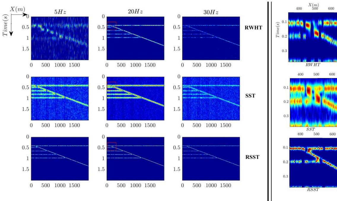
**Figure 3.** Wedge model example. (Left panel): The results of the RWHT, SST, and WSST for the mono-frequency components of 5, 20 and 30 Hz. (Right panel): The zoomed view of the red boxes for frequency of 20 Hz.
